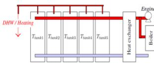
Diagram of the buffer tanks and cogeneration engine
